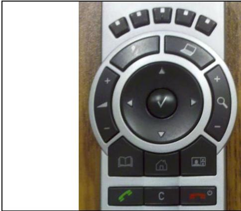
When making selections using the Cisco remote, the various menu buttons have images on them and are arranged in a circle around the arrow buttons. The selection to be chosen within a given menu will display on the screen and will be highlighted on its left side by a light brown bar. Please do not use top row of small buttons on remote. When using the remote, point at the camera, not the codec box.
